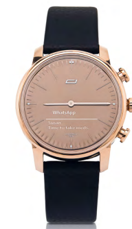
Dayton Industrial's Link2Care Smartwatch DA13700 features a 3D motion sensor to record activity and inactivity, sleep and falls
